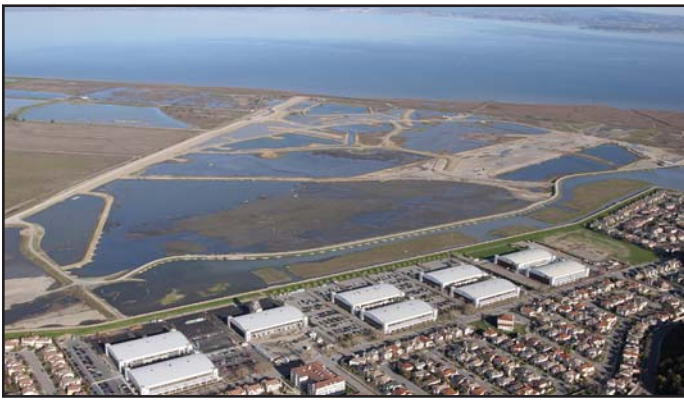
At the Hamilton Wetland site, material is pumped into seven cells to create the proper elevation for a marsh. The hangars in the foreground, from the former Air Force Base, have been converted into office space. Photo: Mark DeFeo/Aerialsondemand.com
